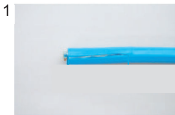
Expose inner vinyl sheath.
